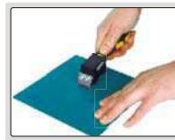
step 1: make grid cutting on surface
